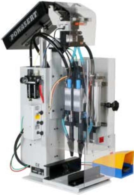
The model ADS-DE1/1 is a stationary twin screwdriver unit with two separate advancing units and integrated screw feeder e.g. to fix the reinforcement in two PVC profiles at the same time.
